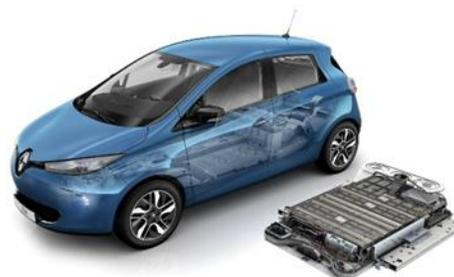
**Zoé** 400 V, 41 kWh, 12 modules, 192 cellules, 290 kg
